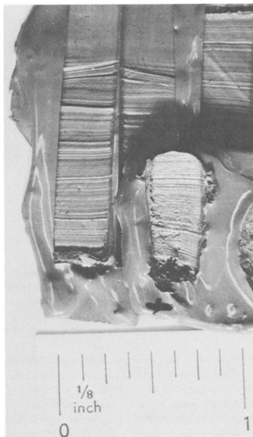
FIG. 5—Coe-Flex "casts" of the suspect knife and cartilage faces. 1 in. = 25.4 mm.
